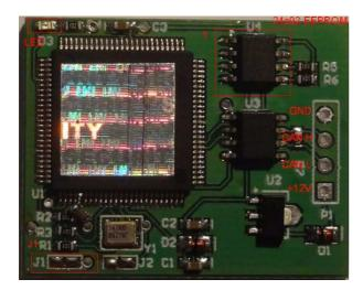
to install Emu you have to solder 4 wires and program 24c02 EEPROM (on Emu Board). File is available from us & program which will create file for 24c02.
